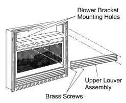
Figure 16 - Removing Upper Louver Assembly
